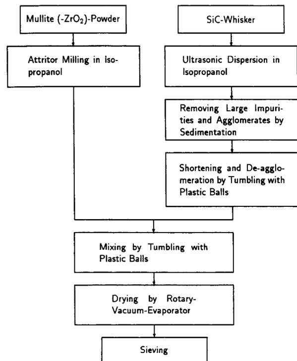
**Fig. 2.** Flow chart of powder processing B.
