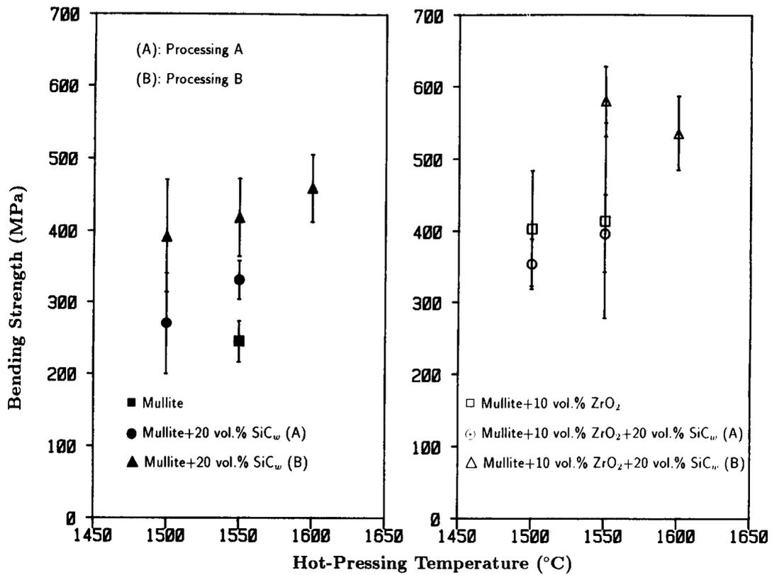
Fig. 5. Room-temperature bending strength of mullite, mullite-matrix composite with 20 vol% SiC whiskers, mullite with 10 vol% ZrO<sub>2</sub>, and mullite-matrix composite with 10 vol% ZrO<sub>2</sub> and 20 vol% whiskers as function of powder processing and hot-pressing temperature.
