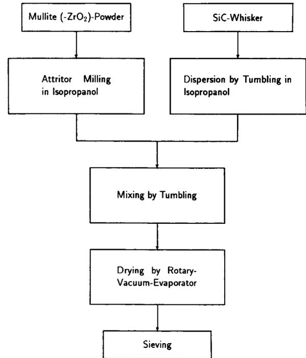
**Fig. 1.** Flow chart of powder processing A.
